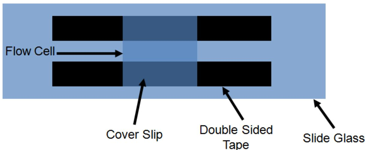
A 100 $\mu$ m thick and ~3mm wide channel will only require ~5 $\mu$ l of volume to fill.
